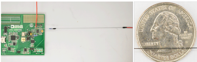
Figure 8: Our thread sensor prototype, coupled with a 470k \Omega resistor and connected to the AD5933 impedance sensing board.
